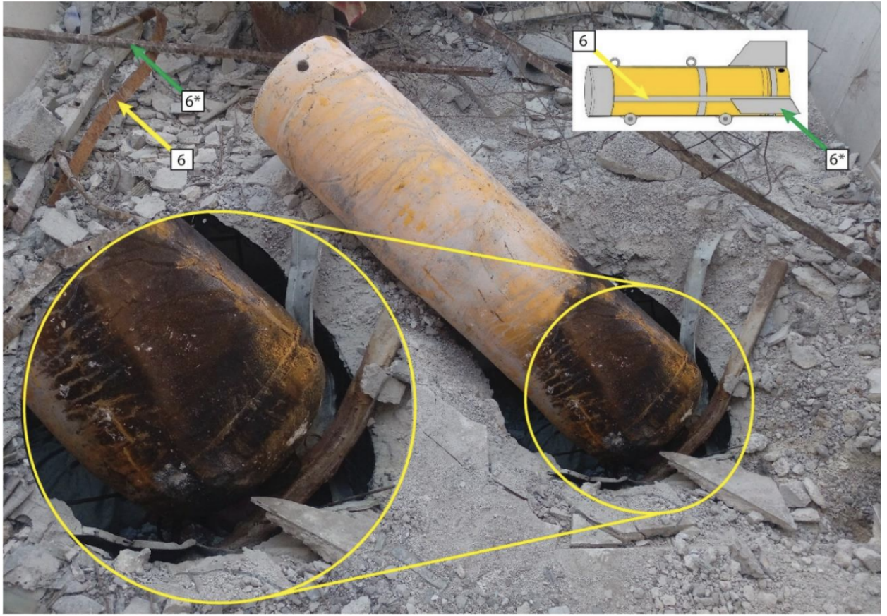
FIGURE 13: THE PATTERN OF DRIED-UP CONDENSATION DROPLETS IS MARKED BY A YELLOW SQUARE (SOURCE: FFM)
